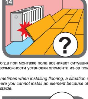
It's necessary to leave an installation and deformation clearance: not less than 10 mm from the edge of covering to the walls. Installation of laminate flooring should be started from laying of the 1st row. Plates are jointed by the edge at the angle of 15 degrees.
